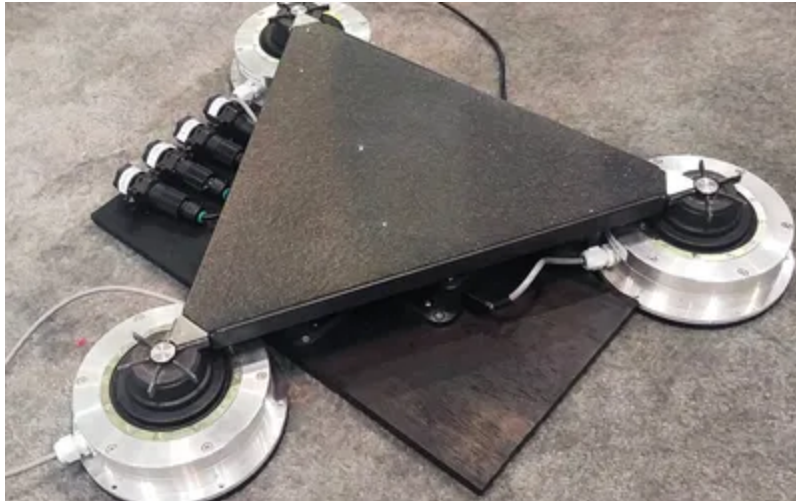
Figure 3A: Pavegen's Version 3 (V3) and most recent tile design [Wevolver, 2023].
